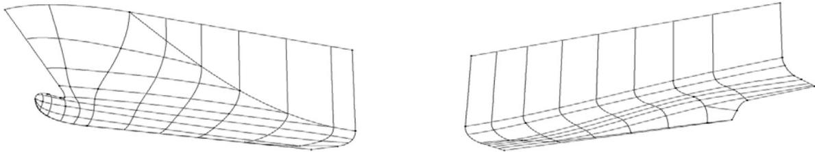
Figure 3: Definition grids of the fore- and aft-body of a typical RoPax ship
