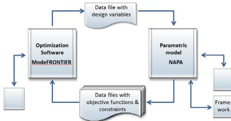
Figure 2: Graphical representation of the optimization setup to be developed and applied in WP5 is presented
