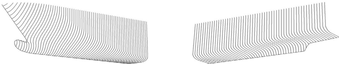
Figure 4: Transverse sections of the fore- and aft-body of a typical RoPax ship
