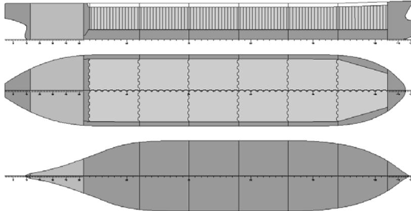
Figure 7: Internal layout of an AFRAMAX tanker with 6 x 2 cargo tanks, corrugated bulkheads and constant double-bottom height
