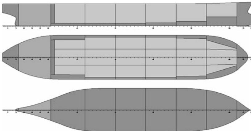
Figure 8: Internal layout of an AFRAMAX tanker with 6 x 3 cargo tanks, planar bulkheads and stepped double-bottom and inner hull
