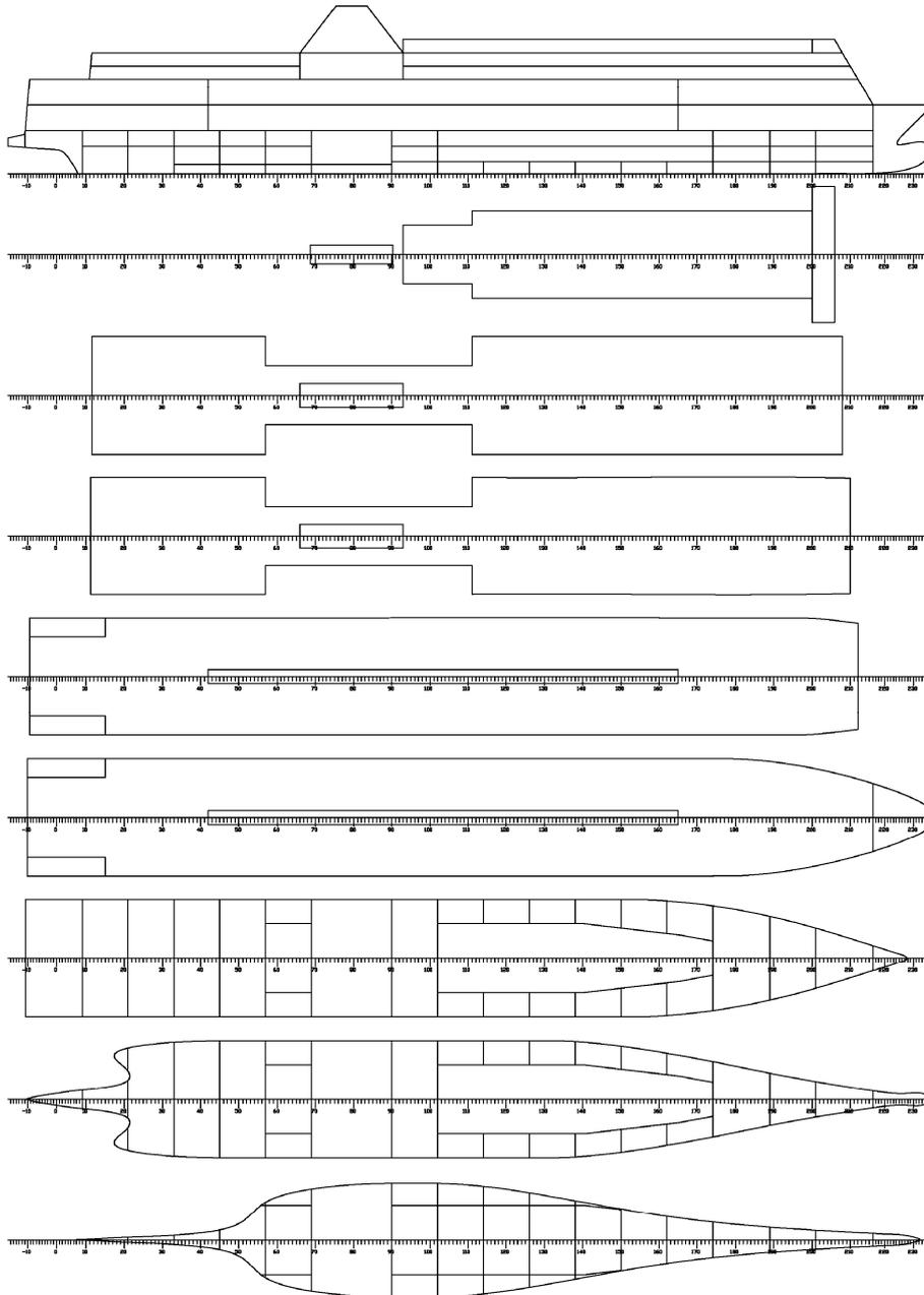
Figure 6: Typical GA of a large RoPax vessel
