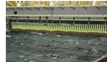
Snake-typed wave maker at NRIFF
