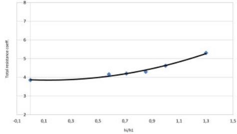
Figure 4. Grid convergence of the total resistance.
