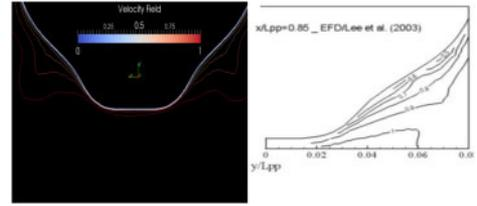
Figure 10. Velocity field at  $x/L_{pp} = 0.85$  (Left-OpenFOAM, Right-Experimental).
