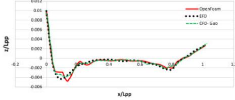
Figure 6. Free surface wave elevation along the hull.
