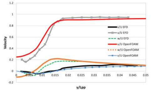
Figure 11. Velocity profile at propeller position along  $z/L_{pp} = -0.05075$ .
