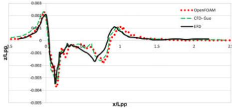
Figure 7. Wave profile at  $y/L_{pp} = 0.0964$ .
