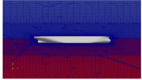
Figure 1. Grid around KVLCC2 hull.
