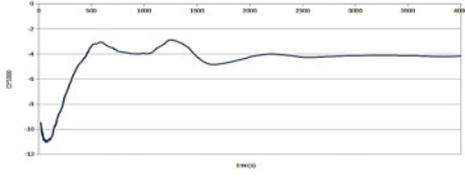
Figure 5. Ship resistance coefficient time history for case 1.
