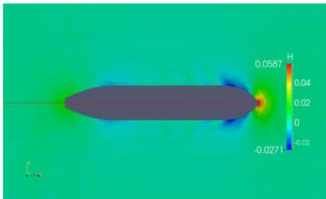
Figure 12. Wave pattern in calm water,  $Fn = 0.142$ .
