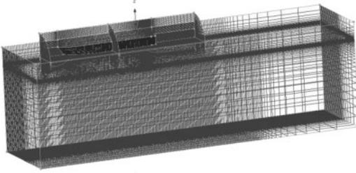
Figure 3. Overset mesh structure for SHIP\_Motion.
