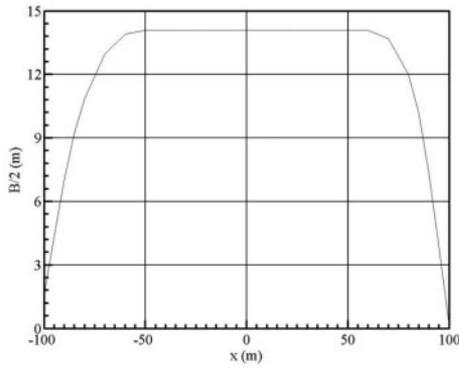
Figure 1. Half breadth at each station in meters.
