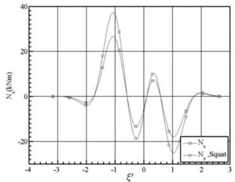
Figure 5. Interaction moment acting on the ship in encounter manoeuvre, with and without accounting Squat.
