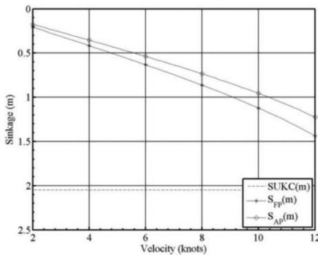
Figure 3. Ship sinkage at bow and stern versus velocity.
