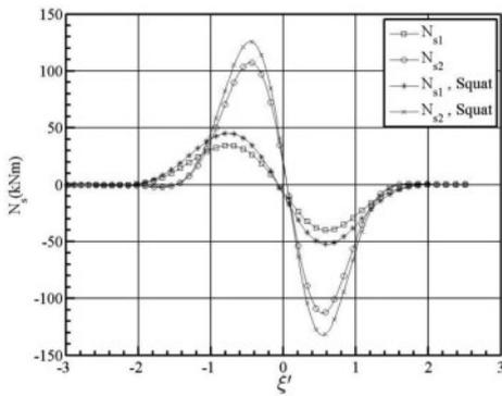
Figure 7. Yaw interaction moments acting on ships 1 and 2 in overtaking manoeuvre, with and without accounting squat.
