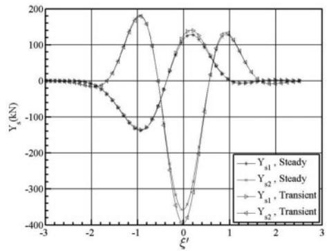
Figure 9. Sway interaction forces with and without accounting for back influence of close-proximity manoeuvres on squat.
