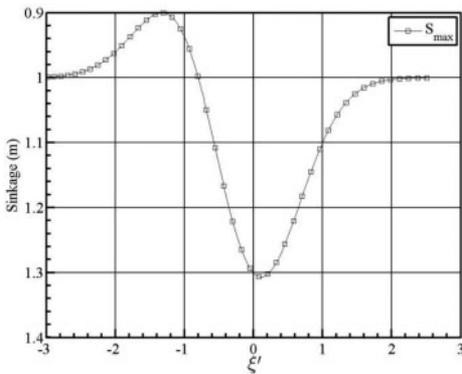
Figure 8. Sinkage at the bow due to close-proximity manoeuvres.
