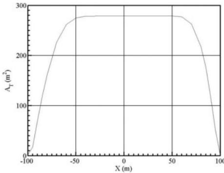
Figure 2. Sectional area curve.
