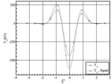
Figure 4. Interaction force acting on the ship in encounter manoeuvre, with and without accounting squat.
