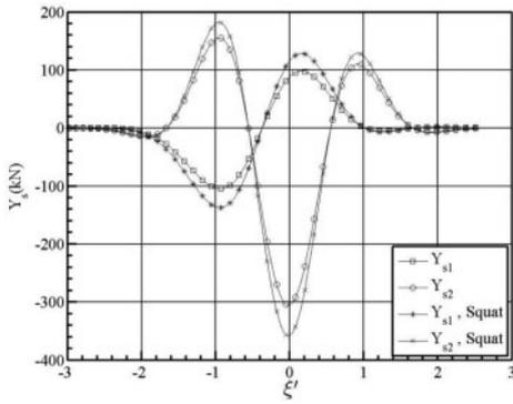
Figure 6. Sway interaction forces acting on ships 1 and 2 in overtaking manoeuvre, with and without accounting squat.
